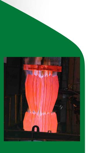
*Kverneland 12 hours carburising process results in creating 2 steels in 1 sole mouldboard.*
