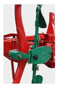
The Kverneland 2500 i-Plough® features legs with a new design, called "aero-profile". Not only higher than the standard Kverneland legs, these new legs improve the soil flow. Heavy residues are pushed out, hence limiting possible blokages regarless of the 85/100 cm interbody clearance.
