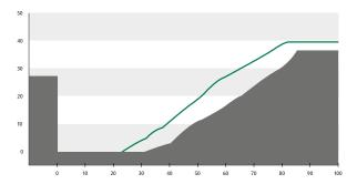
furrow profile body No. 28 working depth: 26 cm, buttom: 30 cm, width 73 cm
