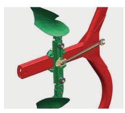
For the perfect ploughing, adjusting the depth of the skimmers is important. Uncorrect adjustment of skimmers causes unfavorable placement of residues in the ploughed soil. This new solution contributes to making ploughing more efficient.
