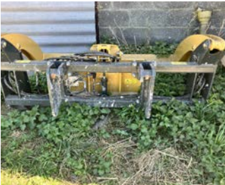
2024 Tanco 173 BALE SHEAR Ref. AG31553 C/W – Manitou Headstock, 1.82m wide, splits bales up to 1.55m diameter, retains plastic wrap. Max of 3 bales cut.
