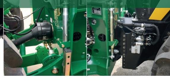
The Twiga Flex series is available with four alternative mounting options for stable and safe performance. Heavy duty and high strength in design, your Twiga can be easily mounted in minutes.
